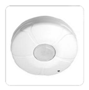
A-ES3: 360° Stand Alone Type Motion sensor is a fully automatic indoor and outdoor security/courtesy light controller capable of controlling up to 1000W incandescent or 30W x 10 fluorescent of lighting. At night, the built in passive infrared (PIR) motion sensor turns on the connected lighting system when it detects motion in its coverage area. During the day, the built in photocell sensor saves electricity by deactivating the lights.
