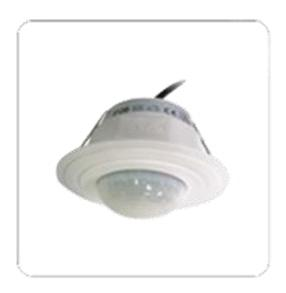
A-ES7: 2000 W Occupancy detector, 360° micro motion detector, Ceiling flush mount, Photo sensor inside for smart control, Run-on time adjustable Ambient lux. setting adjustable, Up to 1500W loading for fluorescent (T8), Smart RelayTM inside to protect product life.
