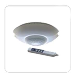
A-ES9: 2000 W 360° ceiling surface mount Occupancy detector with IR remote controller, 360° micro motion detectable, Ceiling surface mount design, Photo sensor inside for smart control, Run-on time adjustable, Ambient lux. setting adjustable, Up to 2000W loading, Smart RelayTM to protect product life, Support IR remote control for On/Off/Auto Control.
