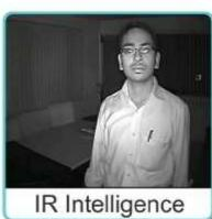
Auto adjusts IR intensity based on the object proximity, for clear face identification
