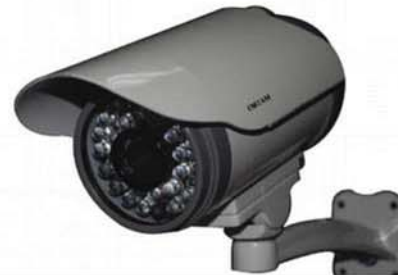
UC-IPSO52C-IR IP IR Outdoor Camera 1/3 Sony Exview CCD 520TVL
