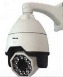
UC-IPSO52C-IR IP IR Outdoor Camera 1/3 Sony Exview CCD 520TVL
