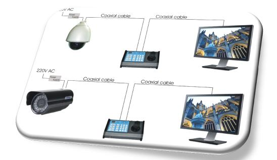
Multiple *Coax-Con* Camera (*BE-6060CV & BE-1806i*) connectivity with *Coax-Con unit.*
